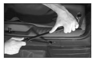
To remove the underbody-mounted spare, insert the socket end of the extension on a 45° angle downward into the hoist drive shaft hole. It is exposed when the rear gate is open and is just above the rear bumper. Be sure the socket end of the extension connects to the hoist shaft. Turn the wheel wrench counterclockwise to lower the spare tire. Keep turning the wheel wrench until the spare tire can be pulled out from under the vehicle.
